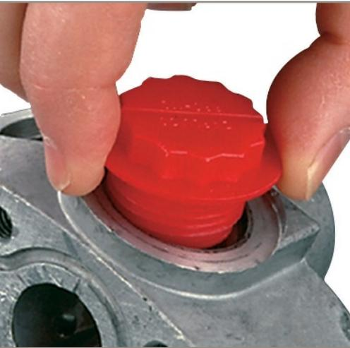
RPO Series plugs provide a positive dual seal on SAE straight-threaded ports. Integral O-ring-type bead seals into bevel of threaded opening to prevent oil or fluid leakage. A lip on the flange compresses against the surface to keep contaminants from the spot face. Easy to install or remove with a slotted 12-point head for screwdriver, socket or wrench tightening.
