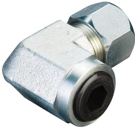
TH Series plugs are designed to protect internal threads during low-pressure testing and in-plant process. Safely keeps contaminants and moisture from threaded ports. Oil and heat resistant to 250°F. Not intended for permanent applications.
