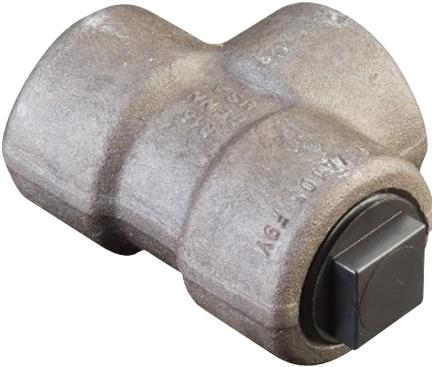
TPN Series plugs are ideal for low-pressure testing and in-house handling. The square-head design enables easy installation. These plugs protect threaded ports from damage, contamination and moisture. Resistant to oil and heat up to 250° F. Not intended for permanent applications.
